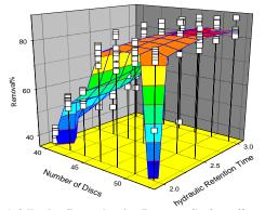
Fig. 1. following figure showing Response Surface effect of Retention Time and Number of Discs on Removal of Biological Oxygen Demand (BOD<sub>5</sub>)
