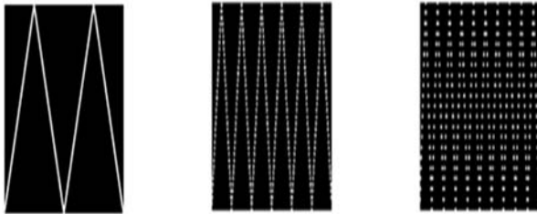
Fig.9. Example of 2 Cycles, 6 Cycles and 10 Cycles Oscillation
