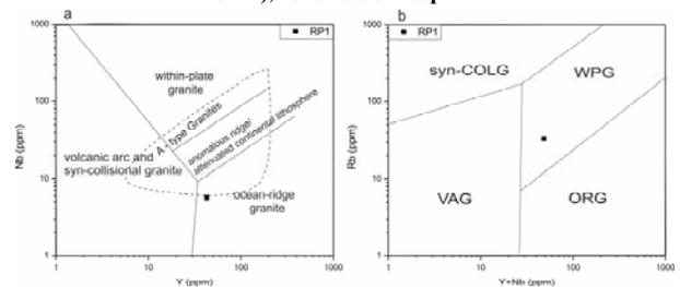
Fig. 3. Discrimination diagrams (a) Y vs Nb and (b) Y+Nb vs Rb, (Pearce, *et al.*, 1984) for the RP1 sample.
