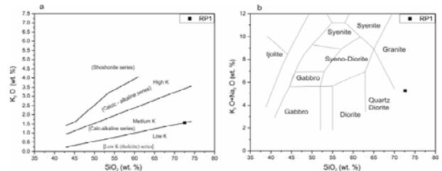
Fig. 2. TAS classification diagram (a) Chemical classification (Wilson, 1989), (b) Total alkali classification (Peccerillo and Taylor, 1976), of the RP1 sample.
