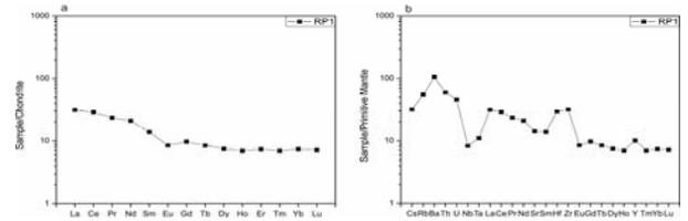
Fig. 4. (a) Chondrite normalized REE diagram (b) Primitive Mantle normalized spider diagram, for the RP1 sample. Normalization values are from Sun and McDonough (1989).
