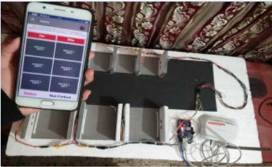
Fig 6. Prototype parking system. The parking slots are all empty but one, which is also shown in the Android app.
