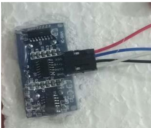
Fig 3. Ultrasonic sensor attached with jumper wires.
