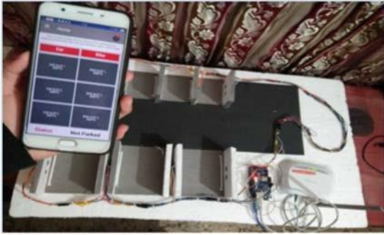
Fig. 5. Prototype parking system. The parking slots are all empty, also shown in the Android app.
