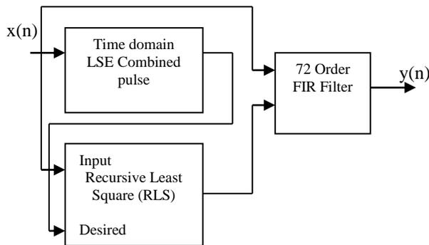
Fig. 15. Workflow for designing RLS filter
