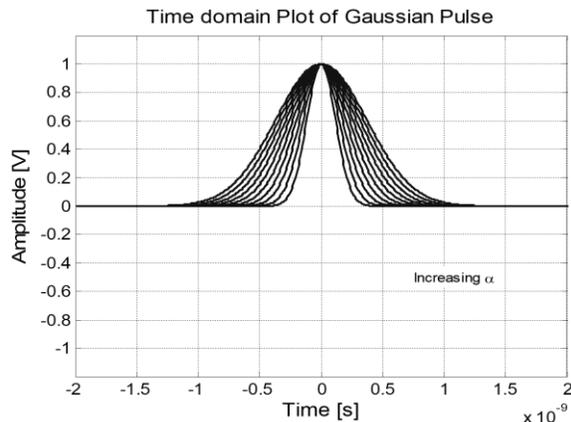
Fig.4: Time domain plot of the Gaussian Pulses with different values of shape factor  $\alpha$ .
