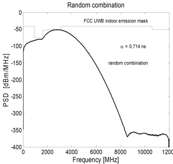
Fig.9: PSD of the Summed Waveform with FCC Constraints
