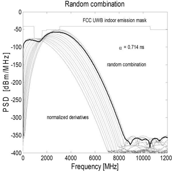
Fig.8: PSD for Derivatives of Gaussian Signal
