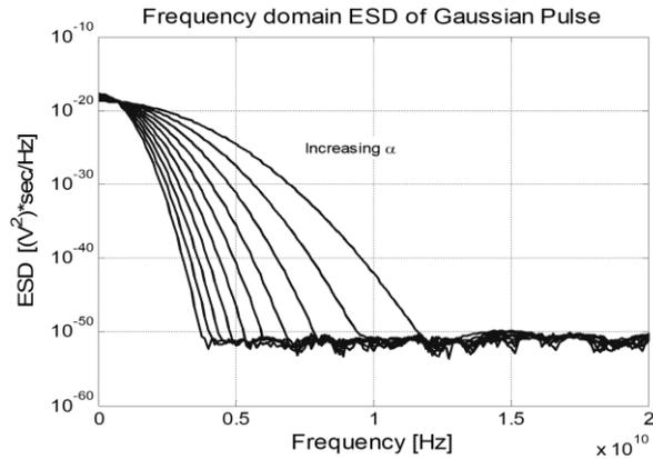
Fig.5: Frequency domain plot of the ESD of Gaussian Pulses with different values of shape factor  $\alpha$ .
