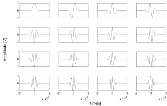
Fig.6: Time Domain plot of Zero to Fifteen Derivatives of Gaussian Pulses from Left to Right.
