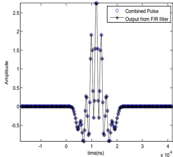
Fig. 16: Comparison of our FIR Filter output and LSE Combined Pulse
