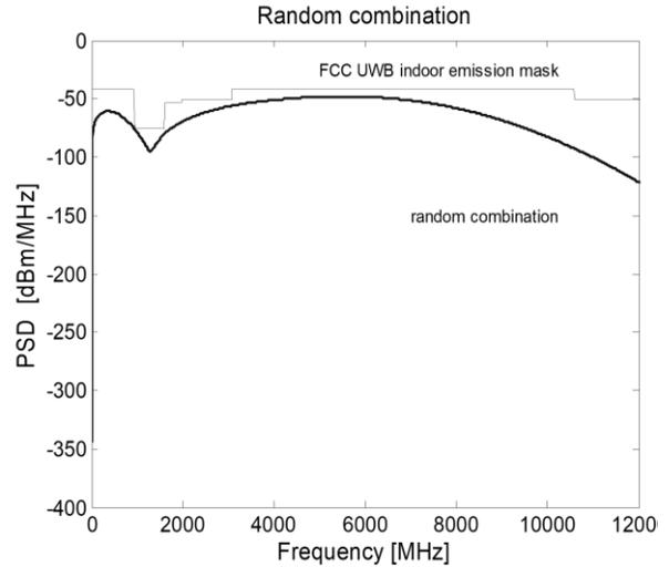
Fig. 11.Frequency Domain Plot of Summed Waveform(PSD) with  $\alpha=1.5$  ns for 1<sup>st</sup> Gaussian Derivative and  $\alpha=0.314$  ns for 2<sup>nd</sup> to 15<sup>th</sup> Gaussian Derivatives. along with the FCC Constraints.
