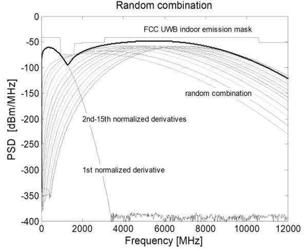
Fig.10: Frequency Domain Plot of Derivatives of Gaussian Pulse (PSD).
