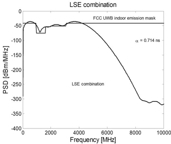
Fig.13: Comparison of FCC UWB Indoor Emission Mask and PSD of Combined Pulses Optimized by LSE.
