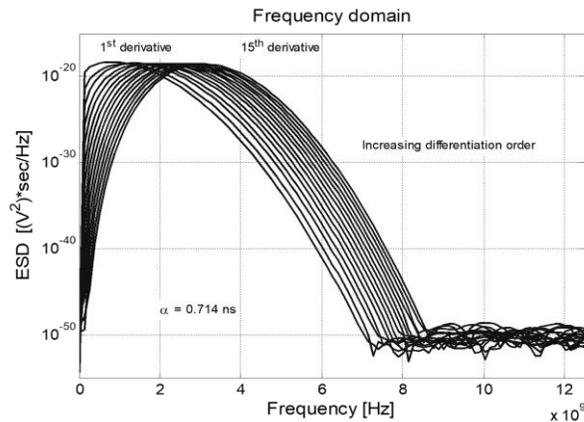
Fig.7: Frequency Domain plot of ESD of Zero to Fifteen Derivatives of Gaussian Pulses from Left to Right.
