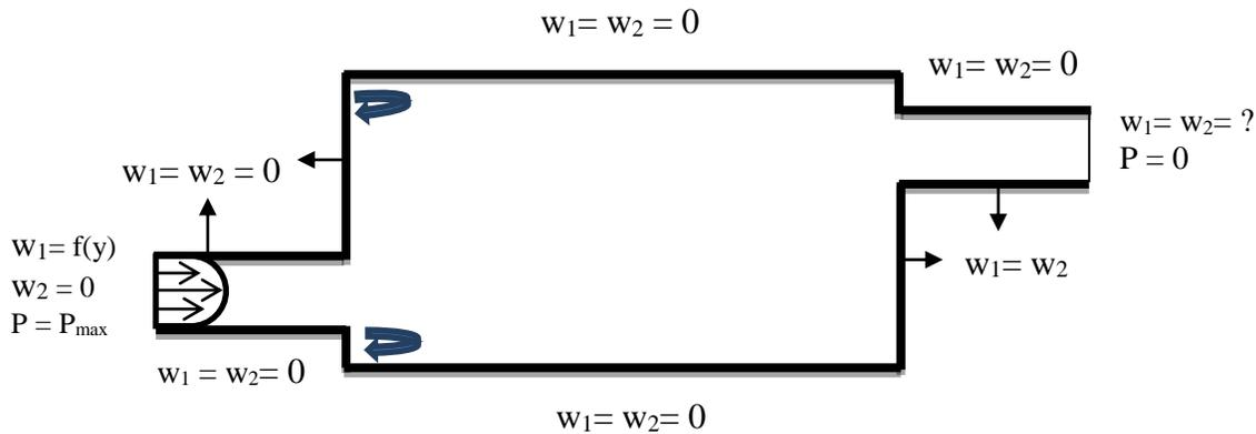
Fig. 1: Schematic Diagram of Converging and Diverging channel
