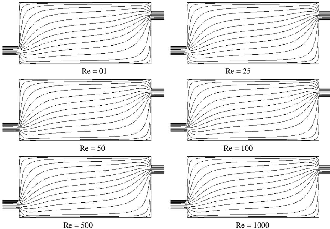
Fig. 5: Two-dimensional Streamlines flow pattern of combined Converging and Diverging channel filled with Pore material
