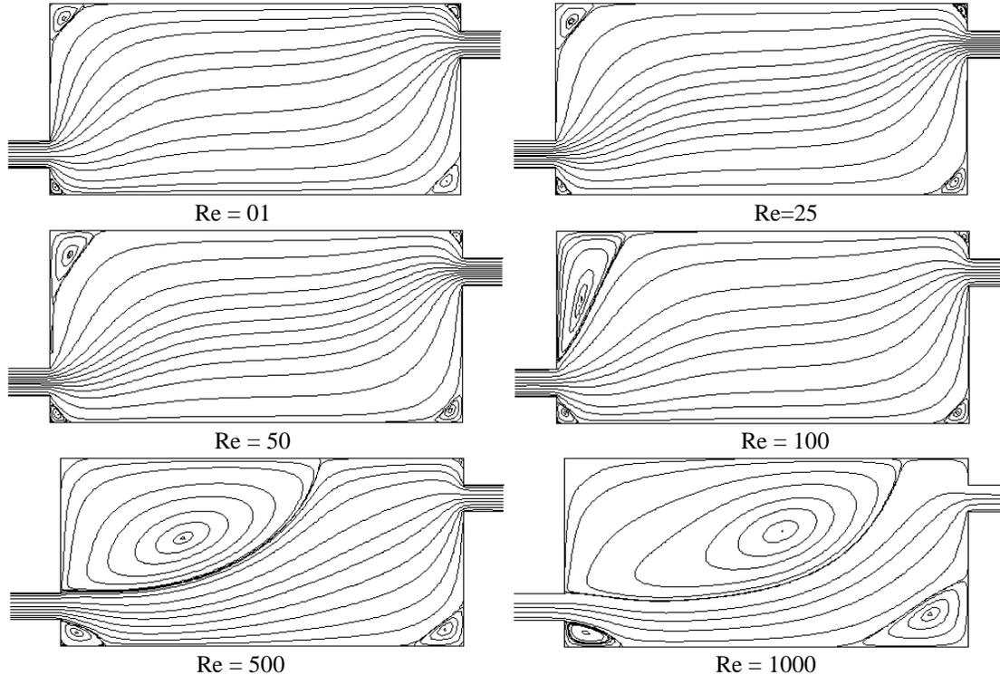
**Fig. 3: Two-dimensional Streamlines flow pattern of combined Converging and Diverging channel.**
