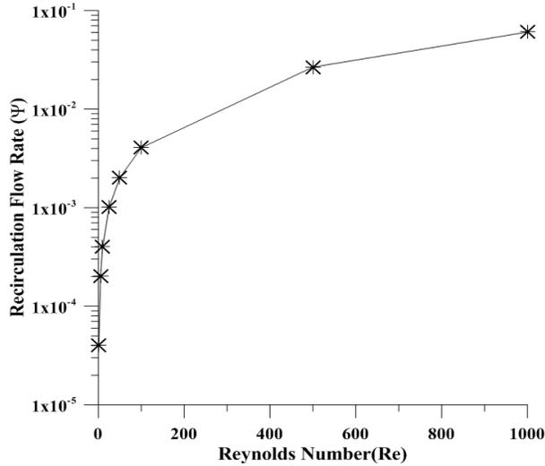
Fig. 4: Graph shows the recirculation Flow rate (RF) on the grows of fluid inertia (Re) forConverging and Diverging channel
