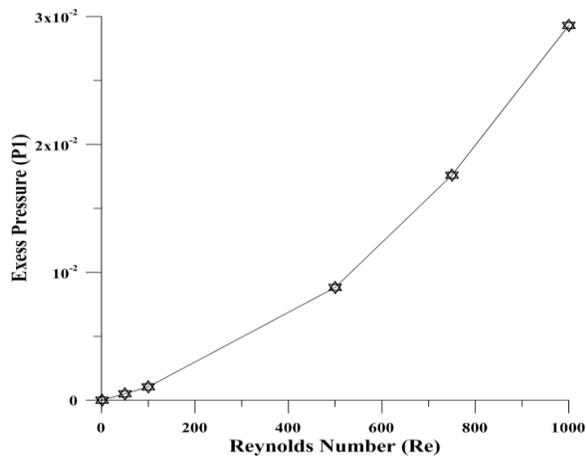
Fig. 6 Excess pressure of two-dimension rectangular channel filled with baffle in terms of the various Reynolds Numbers
