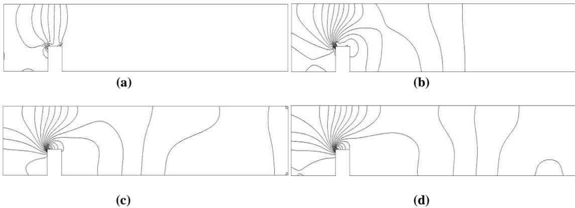
Fig. – 5(a-d): Pressure isobars of two-dimension rectangular channel filled with single baffle in the form of various Reynolds Numbers.
