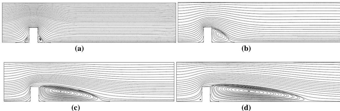
Fig. 3 (a–d):Stream lines for rectangular channel fitted single baffle at lower wall
