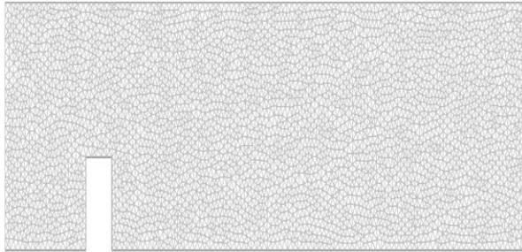
Fig. 2: Extremely fine mesh of two–dimension rectangular channel fitted with single baffle
