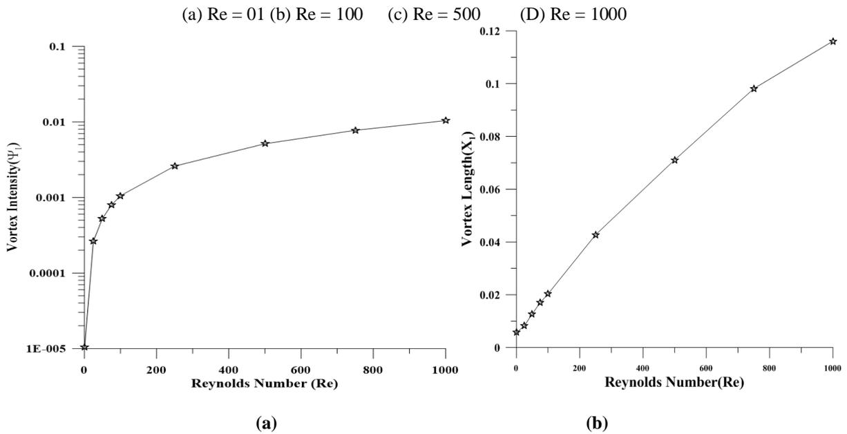
Fig. 4(a-b): Vortex intensity and Vortex Length of two-dimension rectangular channel filled with baffles in terms of the various Reynolds Numbers .
