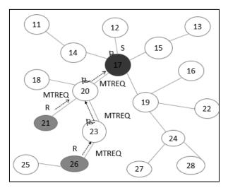
Fig.1. Nodes Receiving Live Data Streams through MTREQ and Forwarding Flag in SLIM+
