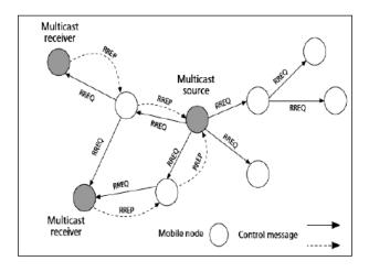
Fig.2. Route Discovery in MAODV Protocol adapted
