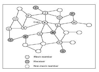
Fig-3. Mesh and Data Forwarding in PUMA adapted
