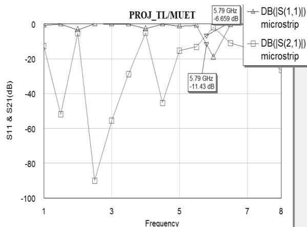
**Fig.10: Microstrip Coupled Line BPF scattering parameters after tuning - Insertion loss (S<sub>21</sub>) and Return loss (S<sub>11</sub>)**
