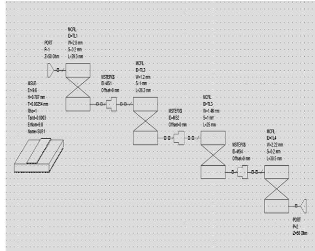
**Fig. 8 :Simulation Model of the proposed microstrip coupled line filter**
