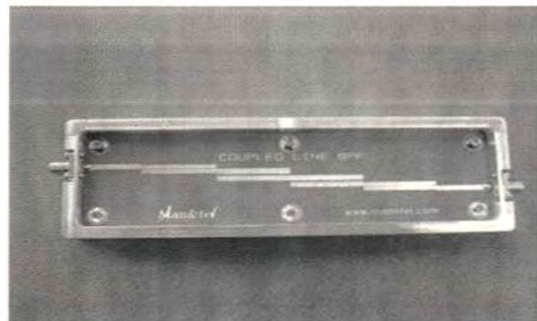
**Fig. 4: Man and Tel's Microstrip coupled line filter**
