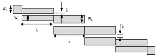
Fig.1: Parallel-coupled, half-wavelength resonator filters
