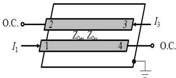
Fig. 2.Coupling sections of dual port filter with propagating channels of current and impedance (odd,even).
