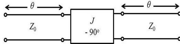
Fig. 3: Coupled line Section amid J-inverters to evaluate the odd and modes
