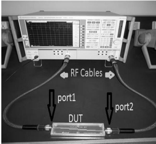
**Fig 5 : Measuring high frequency parameters of Microstrip filter via R&S®ZVA24 Vector Network Analyzer at ADC TL-102 Lab. Mehran UET, Jamshoro.**
