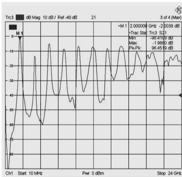
**Fig. 6: Insertion loss (S<sub>21</sub>) of Microstrip coupled filter at 2 GHz**
