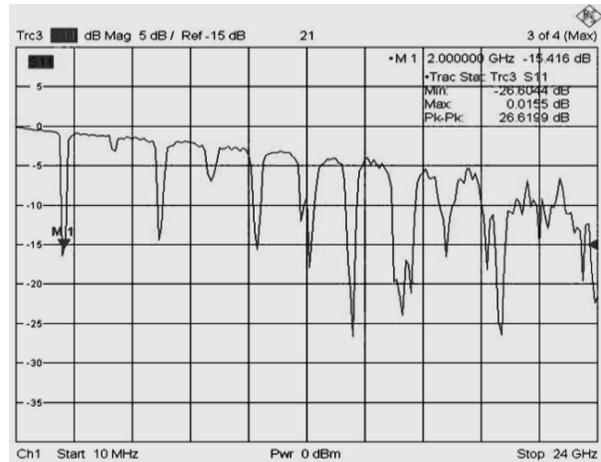
**Fig. 7: Return loss (S<sub>11</sub>) of Microstrip coupled filter at 2 GHz**
