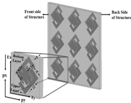
Fig. 1. Geometry of the unit cell and compact four-band circular polarizer based on 3x3 array
