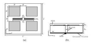
Fig-1 Geometry of Antenna (a) Top view (b) Side View
