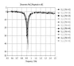
Fig-6 Variation in the S11 parameter with change in the area of patches
