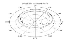
Fig-13 Optimized maximum directivity of reconfigurable antennaat phi=0\*
