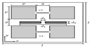
Fig-8 Geometry of Reconfigurable Patch Antenna
