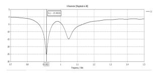
Fig-9 Return Loss when one of switch is ON
