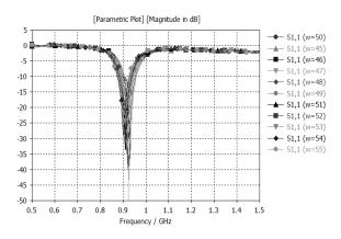
Fig-5 Variation in the S11 parameter with change in the area of substrate
