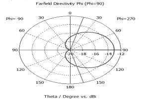
Fig-4 Antenna directivity in H-Plane (maximum at  $E_{\varphi} = 90^{\circ}$ )
