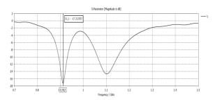
Fig-10 Return Loss when Both Switches are in ON states
