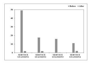
Fig. 3: Oil and Grease Contents in the Washoff Water Before and After Treatment.
