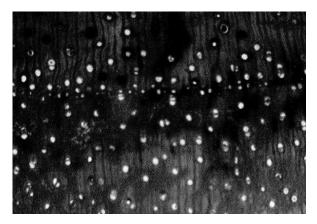
Fig-3 Cross section showing general distribution of Vessels X40
