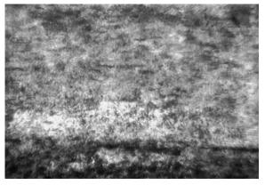
Fig.5 Tangential longitudinal section showing uniseriate rays X100
