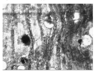
Fig.4 Cross section showing the nature of Vessels and Parenchyma X100
