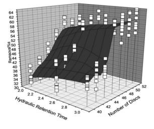
Fig. 1. Response Surface effect of Retention Time and Number of Discs on Removal of Chemical Oxygen Demand
