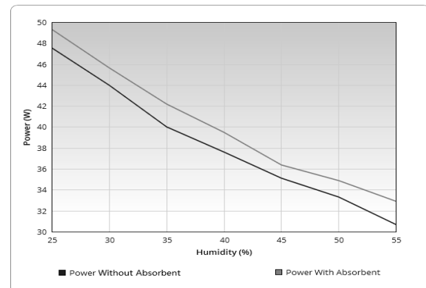
Fig. 3. Influence of Humidity on Power output of a Solar Panel
