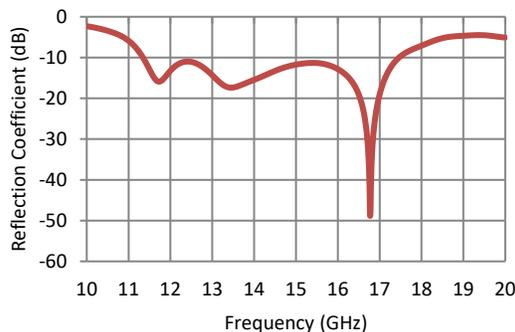
Fig. 3: Return Loss of the proposed antenna
