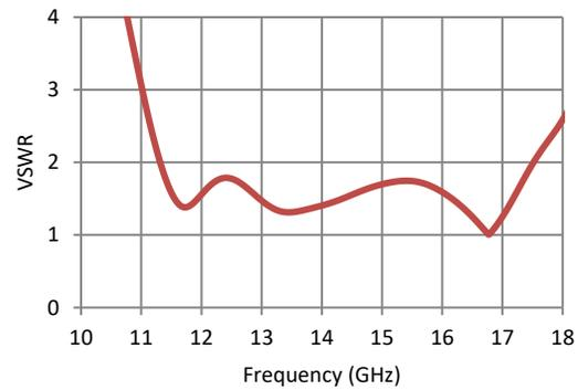
Fig. 4: Voltage Standing Wave Ratio.
