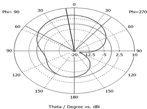
Fig.6b. Radiation Pattern at 13GHz
