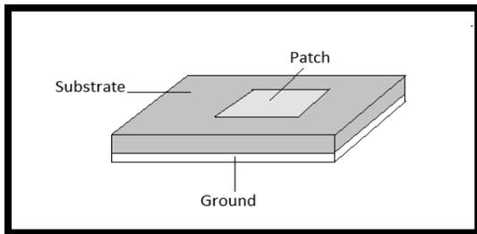
Fig.1. Patch Antenna
