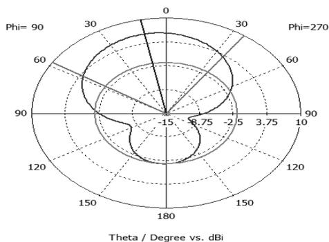
Fig.6c. Radiation Pattern at 14GHz
