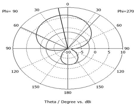
Fig.6d. Radiation Pattern at 15GHz
