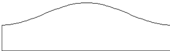
Figure-01: Computational domain for flow interest through Pore-Throat Tube.
