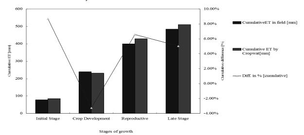
Fig.2 Comparison of cumulative ETo measured in field and calculated by Cropwat.
