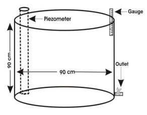
Fig. 1 Schematic layout of the container
