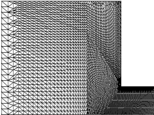
Fig-2: Refined Finite Element Mesh (M) for two dimensional 1:4 geometry
