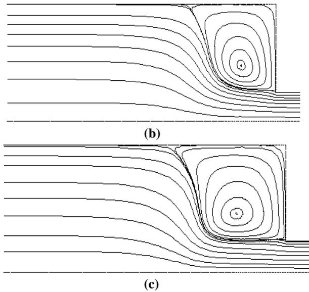
Fig.3: (a – c): Stream lines for 1: 4 expansion flow through pipe.
