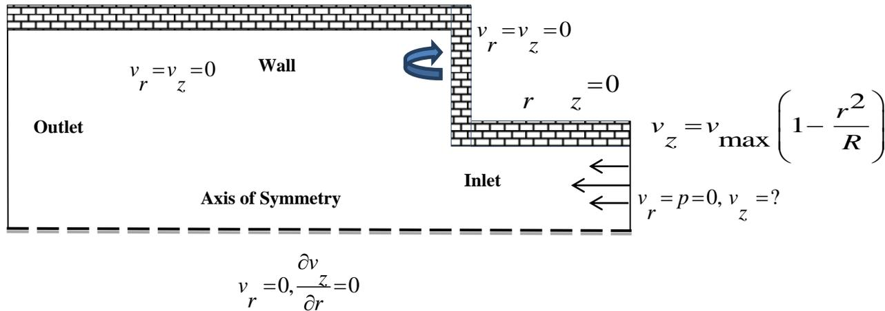
Fig-1: Schematic diagram 1:4 planner expansion pipe with boundary conditions.
