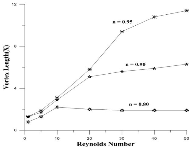
Fig-5: Graph of the vortex cell size (X) is a function of Reynolds Number (Re)
