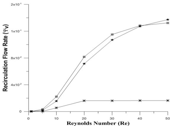
Fig.4: Two dimensional expansion flows, recirculation flow rate (Vortex intensity)( $Q_v$ ) is a function of fluid inertia (Re)
