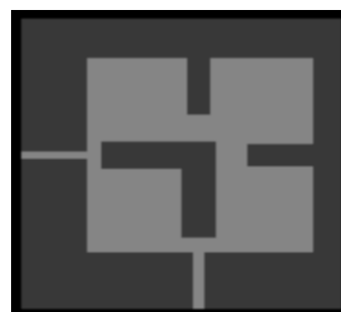
Fig. 15. Filter Layout, input lines directly coupled to the resonator.
