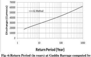
Fig-6:Return Period (in years) at Guddu Barrage computed by Generalised Logistic (GL)method.
