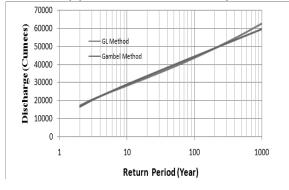
Fig-7: Computed Return Period (in years) at Guddu Barrage by both Generalised Logistic (GL) and Gambel Methods.
