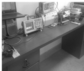
Fig. 8: Experimental setup for Transceiver Design2 (Link distance up to 4 feet)
