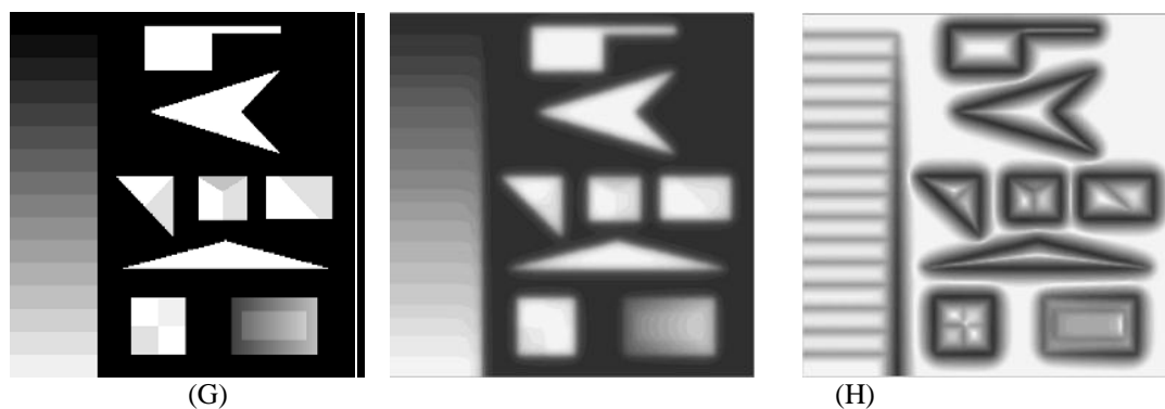
Fig. 3. (G) Original Image with angles and corners (H) Smoothed image using given approximation model (I) Image Segmentation of original image without noise (Edge function v ).
