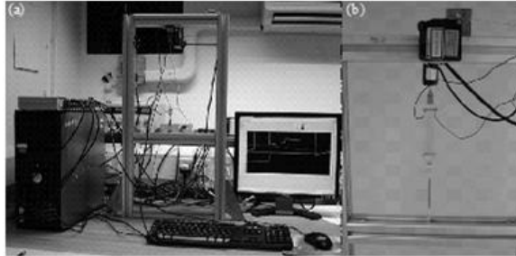
Fig. 1. (a) Instrumented test rig; (b) Bundled actuator mounted on the test rig.
