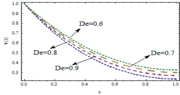
**Fig. 3:** Effect of  $De$  on velocity field, when  $m = 15, \xi = 0.01, S_i = 1.4, Br = 10, \epsilon = 0.01$
