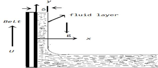
Fig. 1. Physically geometry for fluid flow through vertical belt, which is moving through container.
