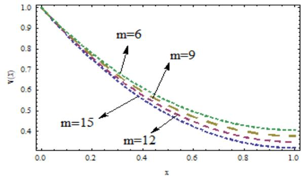
**Fig. 5:** difference of  $m$  on velocity distribution, when  $\epsilon = 1, \xi = 0.01, S_i = 1.4, Br = 10, De = 2$
