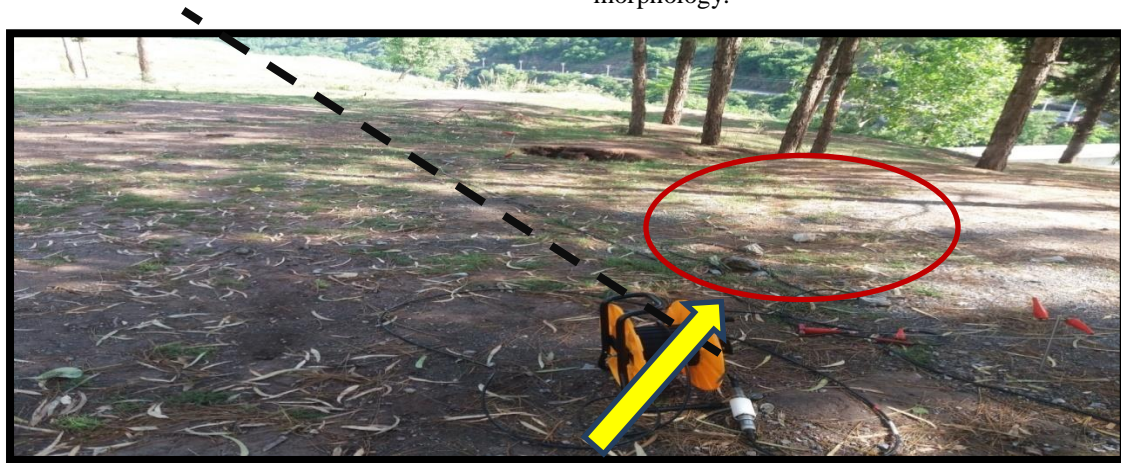
Fig. 5: Resistivity profile line over sinking area.
