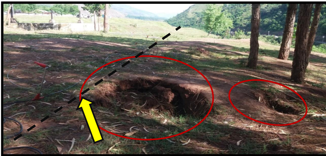
Fig.4: Surface indication of soil sinking.
