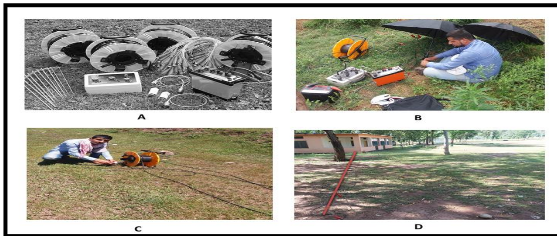
Fig.3: A Instruments use in (ERT) survey. B Field data acquisition system. C Field cables spread. D Field data acquisition line
