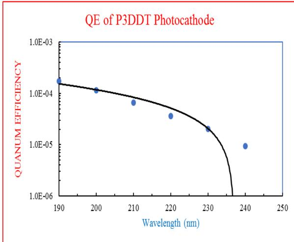
Fig. 2 QE of P3DDT using dissolving in solvent technique
