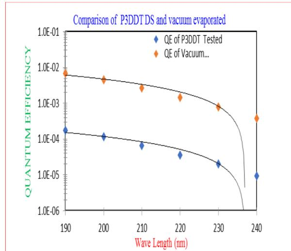
Fig 4 QE of P3DDT DS and shift in QE due to vacuum evaporation technique
