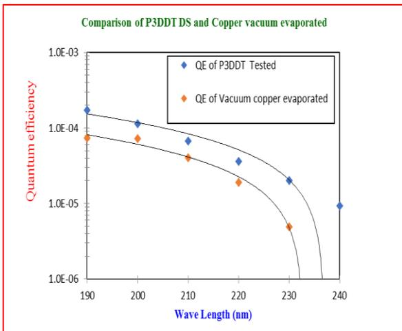
Fig.3 Comparison of QE of P3HT photocathode (DS) with copper vacuum evaporated
