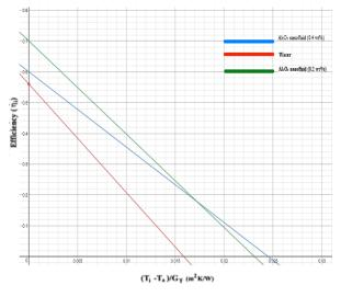
Fig. 1. Comparison of water Vs nanofluid Al<sub>2</sub>O<sub>3</sub> at wt% of 0.2 and 0.4
