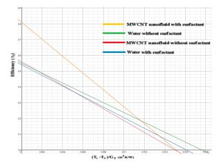
Fig. 4. 0.2 wt% MWCNT nanofluid with and without surfactant vs. water with and without surfactant
