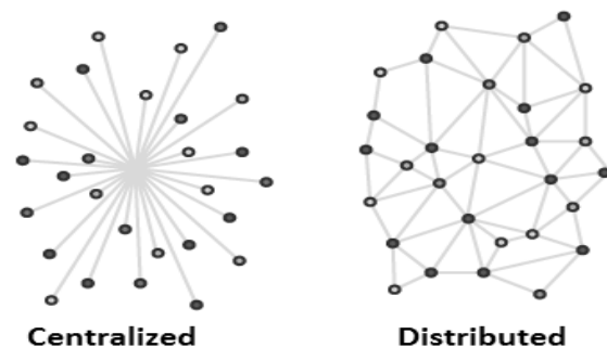
Figure 1: Difference between centralized and distributed
