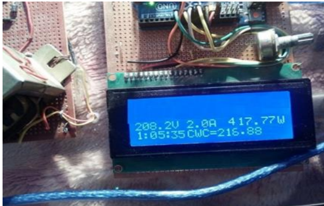
Figure 6. Active Power Load of TV (Television) Smart Hardware Module
