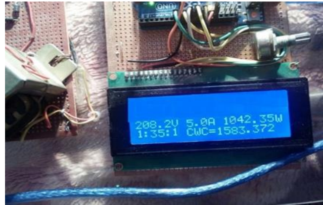
Figure 3. Active Power Load Reading on Smart Hardware Module
