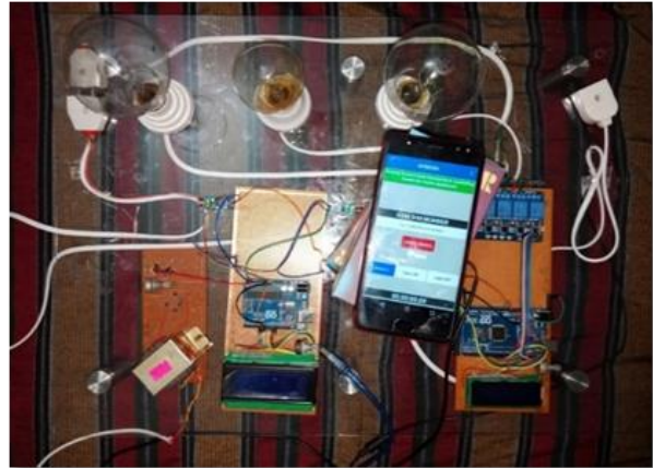
Figure 5. Hardware Component of APMCSH System
