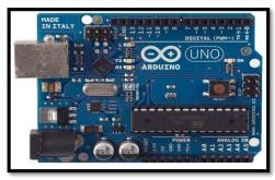
Figure 4. Arduino hardware
