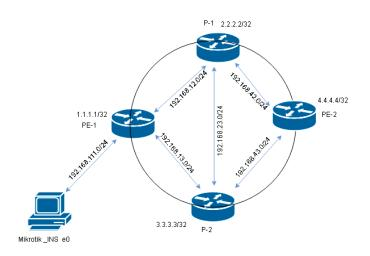
Figure 3: showing the test topology used for the testing of Mikrotik virtual OS and its performance
