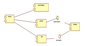
Figure 7: Components composition example in UML 2.0
