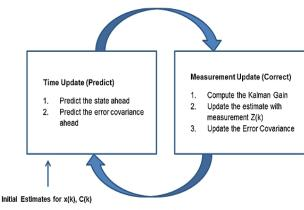
Figure 1: Kalman Filter Process
