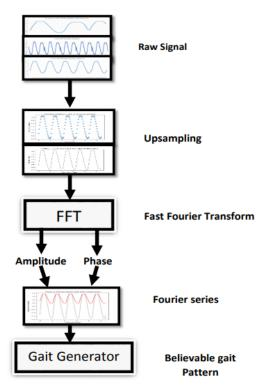
Figure 10: Overview of the analysis process.
